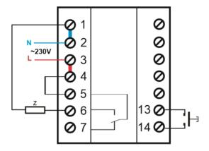
On the above mentioned figure is shown an example wiring scheme, where the consumer  $\mathbb{Z}$  operates with a voltage of ~230V. The bridge between terminals 4 and5 should not be placed, when the consumer operates with a different voltage than ~230V.
