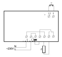
On the above mentioned figure is shown an example wiring scheme, where the consumer Z operates with a voltage of  $\sim 230$ V. The bridge between terminals 8 and 9 should not be placed, when the consumer operates with a different voltage than  $\sim 230$ V.
